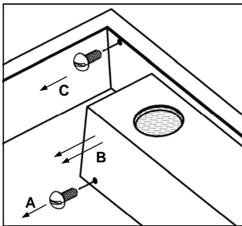
liner to interior of hood shell. Remove screws (C) and set the liner aside.
